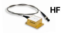
Sheaumann's high heat load (HHL) modules incorporate an internal TEC, thermistor, and photodiode to withstand high heat operation. HHL modules are electrically isolated, hermetically sealed, and can incorporate a variety of options including optics for fast axis collimation. Sheaumann's proprietary laser chip design offers unrivaled quality and long lifetime. Wavelength emission range 780-1070nm. Many fiber-coupled options are available.
