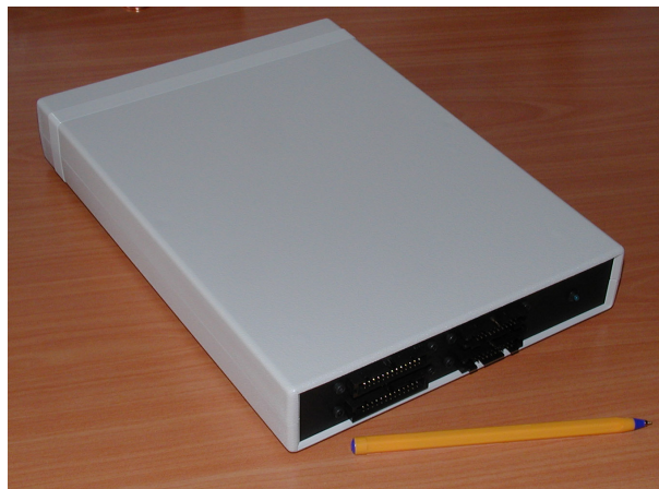
Figure 4: 40 channel high-voltage amplifier unit.
