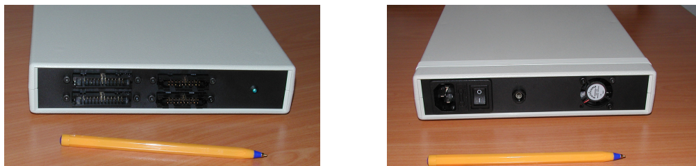
Figure 5: Front and back panels of 40 channel high-voltage amplifier unit.
