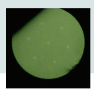
These Ge-doped silica multicore fibres integrates 7 photosensitive cores (6 hexagon-arranged cores around a center core) which make them particularly suited for Bragg grating inscription and sensing application (Shape, Strain, Temperature...) in the C-band. On-demand custom fiber design possible: core numbers, core location and composition.
