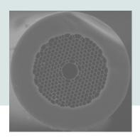
Optical signal in a hollow core photonic bandgap fibre is guided in an air core surrounded by a high air filling factor PBG microstructured region (>90%). Added to the bend low sensitivity due to the core high NA, this confers to this fibre design significantly reduced material nonlinearities since more than 95% of optical power is propagating in air. In addition air/undoped silica provides excellent temperature immunity critical for high performance fibre sensing and metrology applications.
