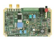
Koheron QCL100 is a high-performance current source designed to drive Quantum Cascade Lasers. With a low current noise of 650 pA/√Hz, the QCL100 driver provides an adjustable compliance voltage up to 15 V at 500 mA and an adjustable precision current limit. The QCL100 driver features a 5 MHz modulation input and a 10 Hz trimming input and is supplied from a single 24 V input.
