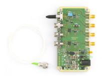
Koheron LPD100 combines a 1550 nm DFB laser (same as LD101), a 100 MHz balanced photodetector (same as PD100B-AC) and a 100 MHz single photodetector (same as PD100-AC). It operates from a single supply voltage ranging from 6 V to 28 V.
