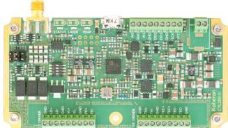
Koheron CTL200-0 is a digital low-noise laser diode driver combined with a TEC controller. It drives up to 600 mA laser current with a compliance voltage up to 3.2 V. It is the screw terminal version of the [CTL200 digital butterfly laser diode controller](#).
