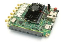
The ALPHA250 is a programmable board built around a Zynq 7020 SoC. It features a 100 MHz RF front end with dual 14-bit ADC 250 MSPS and dual 16-bit DAC 250 MSPS. Analog input to output latency is less than 90 ns. The RF ADC and DAC are clocked by a dual PLL, ultra-low jitter clock generator. It includes a 4 channel 24bit ADC and 4 channel 16-bit DAC. The board comes with a comprehensive, open source, FPGA / Linux reference design.
