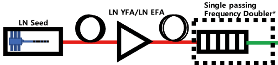
Fig. 1, Schematic of the low noise fiber laser. *The doubler module is equipped with SHG model
