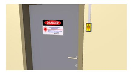
The front door is shown from the exterior. The LSS2380 Warning module will display the status of the room interlock. It will illuminate with red text when armed that can say "Danger, Laser On" or it can simply say "Laser On" if the jumper on the printed circuit board is placed. The yellow laser hazard triangle can be configured to flash as a strobe or remain on solid. When the interlock is not armed, it will show "LASER SAFE"
