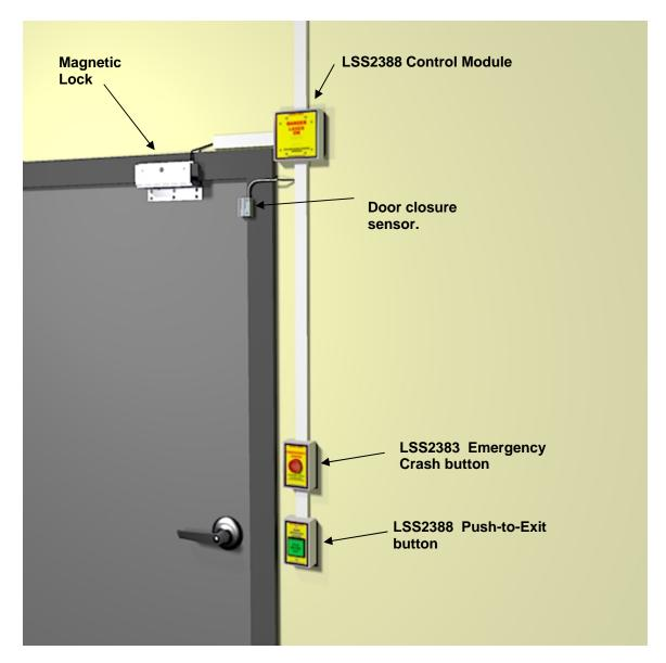
Interior exit is shown above. The door components are installed as described in the LSS2388 User Manual and maglock installation manual. The Push-to-exit module permits egress without tripping the door interlock.
