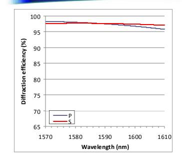
LightSmyth Technologies' transmission gratings are fabricated on fused silica substrates and robust dielectric films by state-of-the-art projection photolithography and reactive ion etch. These high fidelity semiconductor fabrication enable precise methods realization of sophisticated proprietary grating designs that provide diffraction efficiency close to 100% and line spacing control to 1 part per million.
