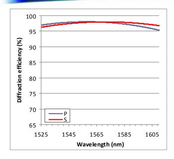
LightSmyth Technologies' transmission gratings are fabricated on fused silica substrates and robust dielectric films by state-of-the-art projection photolithography and reactive ion etch. These high fidelity semiconductor fabrication methods enable precise realization of sophisticated proprietary grating designs that provide diffraction efficiency close to 100% and line spacing control to 1 part per million.
