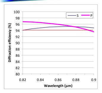
LightSmyth Technologies' transmission gratings are fabricated on fused silica substrates and robust dielectric films bν state-of-the-art projection photolithography and reactive ion etch. These high fidelity semiconductor fabrication methods enable precise realization sophisticated proprietary grating designs that provide diffraction efficiency close to 100% and line spacing control to 1 part per million.
