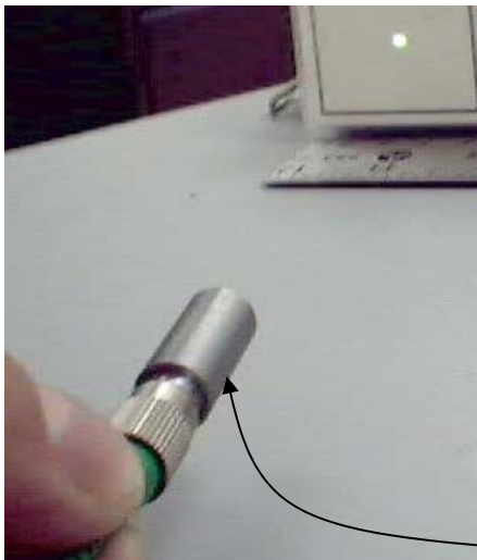
Model 014 focusable fiber collimator
