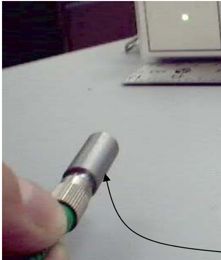
Model 014 focusable fiber collimator
