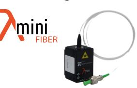
The Lambda Mini Fiber includes an 80 cm single mode optical fiber with an FC-PC or FC-APC connector. The fiber is factory-aligned and permanently attached. Polarizationmaintaining or multi-mode fibers are optionally available. Please contact our sales team for further information.
