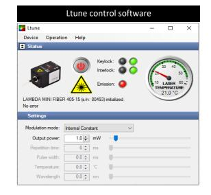
All operating parameters can be monitored and controlled from a PC using the Ltune laser control software for Windows. Alternatively, the laser can easily be controlled from your own application software. Please refer to the user manual for a detailed description of the communication protocol. You can find downloads on our website
