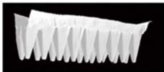
OCT检测3D模型侧视图 Ultrasonic welding joint photo taken by OCT with 3D image.
