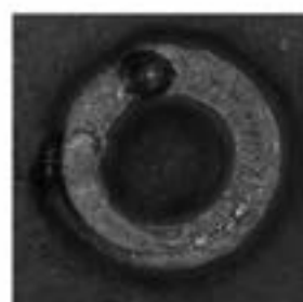
普通相机拍摄铜板焊接轨迹图 Copper plate welding path photo taken by the normal industrial camera.
