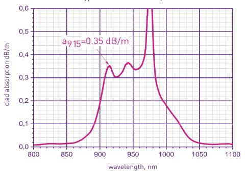
Typical inner clad absorption
