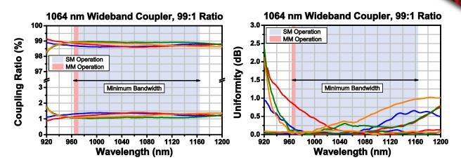
These persistence plots show the coupling ratio and uniformity of four TW1064R1F1A couplers (tap and signal outputs from the same coupler are indicated by matching colors on each graph). The red- and blue-shaded regions denote the coupler's full operating wavelength range. Please note that the red region indicates wavelengths for which single mode operation is not guaranteed, as the cut-off wavelength for the HI1060 fiber utilized in this coupler is  $920 \pm 50$  nm.
