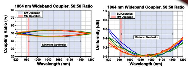
These persistence plots show the coupling ratio and uniformity of four TW1064R5F1A couplers (tap and signal outputs from the same coupler are indicated by matching colors on each graph). The red- and blue-shaded regions denote the coupler's full operating wavelength range. Please note that the red region indicates wavelengths for which single mode operation is not guaranteed, as the cut-off wavelength for the HI1060 fiber utilized in this coupler is 920 ± 50 nm.
