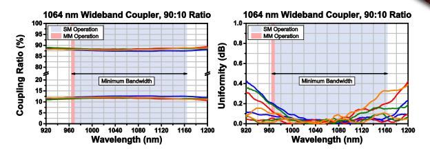
These persistence plots show the coupling ratio and uniformity of four TW1064R2A2A couplers (tap and signal outputs from the same coupler are indicated by matching colors on each graph). The red- and blue-shaded regions denote the coupler's full operating wavelength range. Please note that the red region indicates wavelengths for which single mode operation is not guaranteed, as the cut-off wavelength for the HI1060 fiber utilized in this coupler is  $920 \pm 50$  nm.
