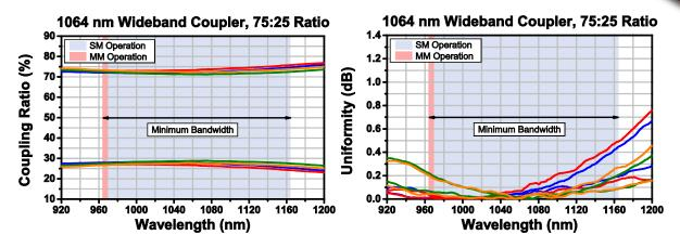
These persistence plots show the coupling ratio and uniformity of four TW1064R3A1A couplers (tap and signal outputs from the same coupler are indicated by matching colors on each graph). The red- and blue-shaded regions denote the coupler's full operating wavelength range. Please note that the red region indicates wavelengths for which single mode operation is not guaranteed, as the cut-off wavelength for the HI1060 fiber utilized in this coupler is 920 ± 50 nm.
