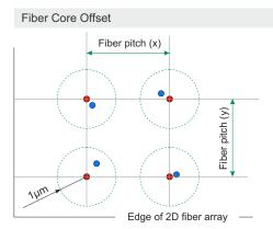
Middle of fiber core - ideal position Middle of fiber core - real position
