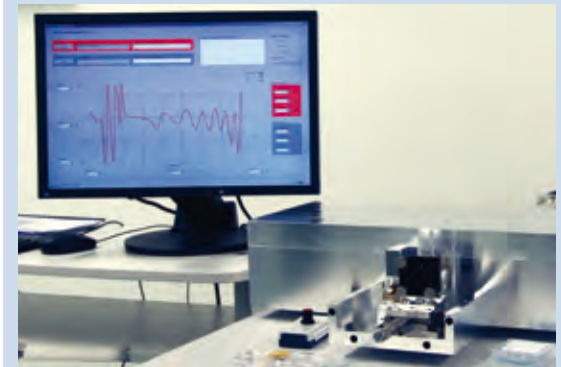
GDD measurement setup
