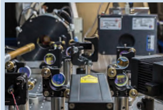
Absorption measurement using a high power cw laser
