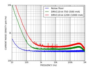
Current noise RMS integrated between 10 Hz and 1 MHz is 168 nA for the 750 mA laser current version (A-750) and 289 nA for the 1200 mA laser current version (A-1200).
