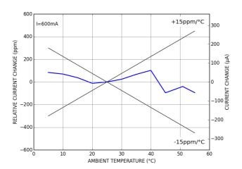
Current stability is depicted in the following figure showing a 24-hour long evolution of current, set to 600 mA at 25 °C ambient temperature. Current is stable within  $\pm 50$  ppm.
