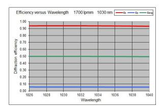
We measure every transmissive VPH grating to ensure exceptional first order diffraction efficiency uniformity over the specified operating band.
