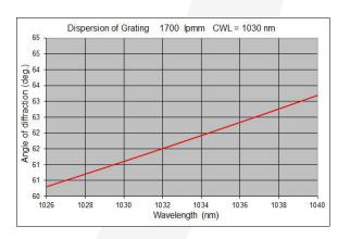
Typical dispersion for a 1700 line/mm VPH grating designed for use at 1030 nm. Custom OEM designs available upon request.
